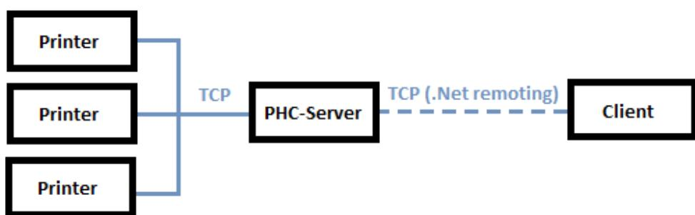
The PHC-Server is communicating with the printer arrays directly on its own network. Any client can connect to the PHC-Server via the “PHCInterface”.
